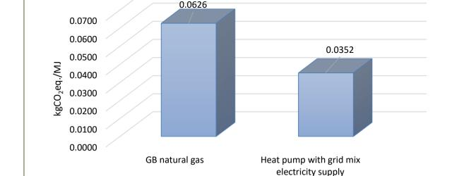
Heat Pump Heat Generation - GB Natural Gas vs Electricity
